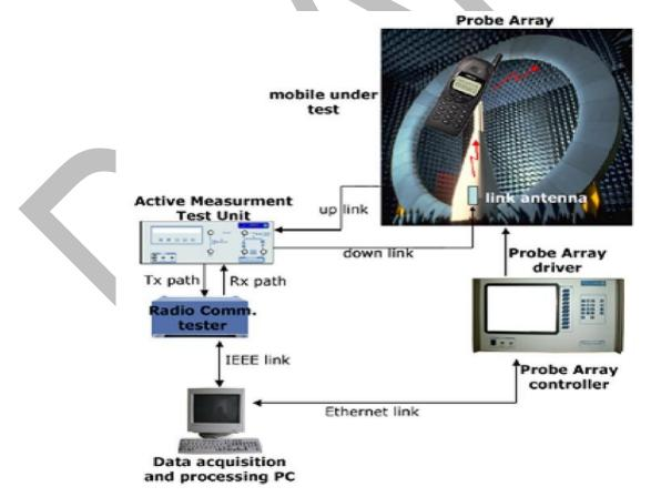
Figure 4-1 SATIMO microwave testing chamber
